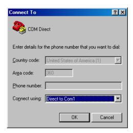
The *COM Direct Properties* window will now appear. Specify *Direct to COM1/COM2* under the *Connect Using* pull-down menu (be sure to indicate the correct COM setting for your system).
