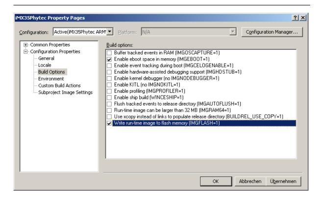
In the Properties dialog select *Configuration Properties* and *Build Options*. Check the "*Write run-time image to flash memory*" and rebuild the solution. Please read Appendix A "How to install Windows CE on the phyCARD-M" for information on how to flash the image.
