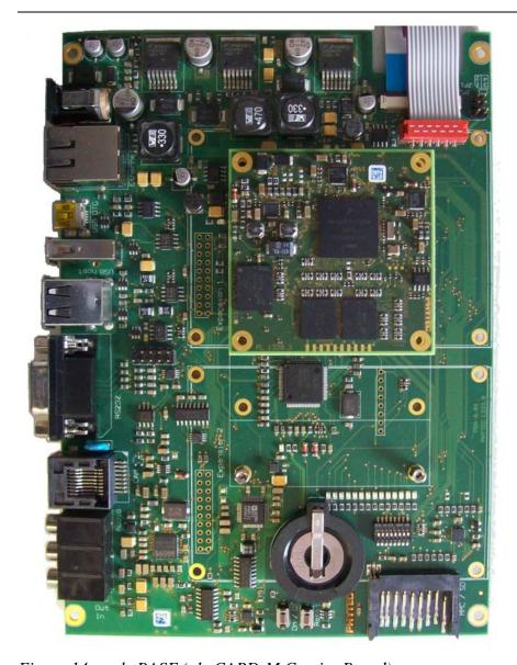
Figure 14: phyBASE (phyCARD-M Carrier Board)
