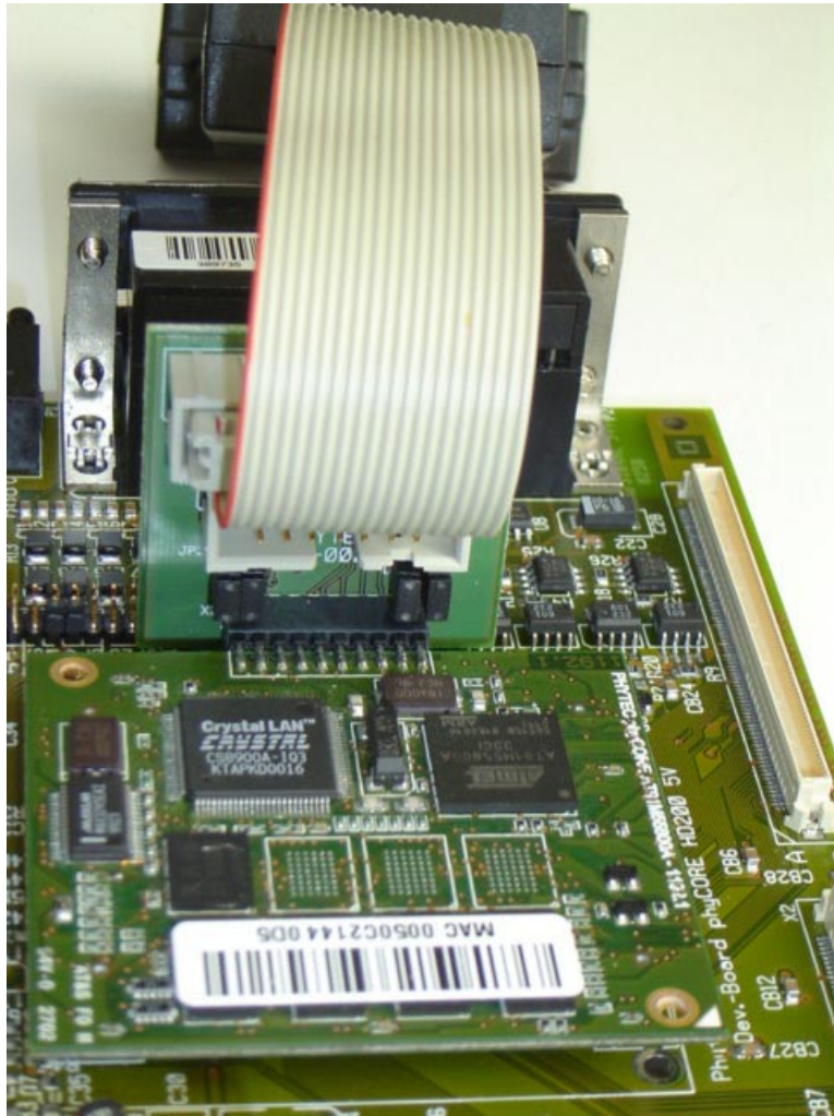
Figure 3: JA-001 and JA-002 Connected to the phyCORE Module
